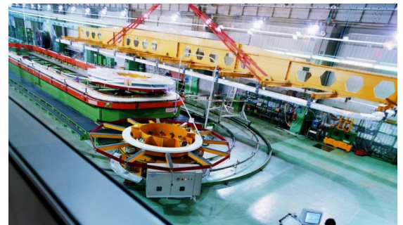
DP winding line and DP translation to the impregnation mould
