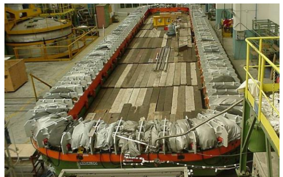
Impregnation mould during DP impregnation cycle
